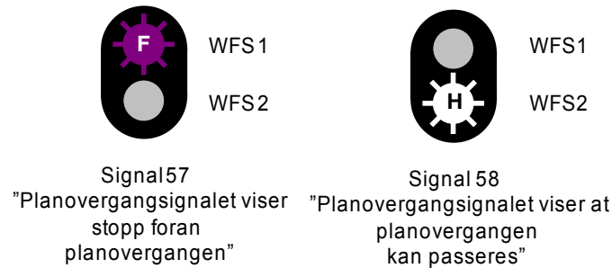
Figur 9.17 Forsignal for planovergangssignal - signalbilder
